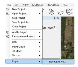
This will open a new window asking for the input.las file. It will also ask if C3D should create a DEM from the .las file and a reference ortho (intensity image). The DEM can be used in lieu producing an autocorrelated surface with C3D. When combined with the intensity image these two outputs can be used to pick GCPs for use with drone imagery and the AT solution.
