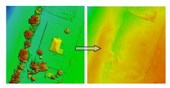
The software analyzes the DSM and removes structures lying on the ground. DTMs are useful for generating orthophotos as they avoid visual artifacts (e.g. along building edges) caused by using DSMs.
