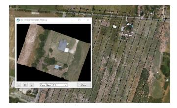
Before an orthomosaic can be generated, individual orthophotos must be created. Orthorectification consists of geometrically correcting the raw images such that they provide an accurate representation of the ground surface. The photos are thus adjusted for topographic relief, lens distortion and camera orientation. Once all orthophotos have been produced, they can be visualized through the software interface.
