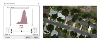
Automatically generated mosaics can be interactively edited using the mosaic editing module. This allows for manual modification of seamlines with real-time visual feedback on the effect of changes
