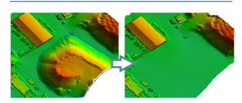
While automatically generated DSMs/DTMs are highly accurate, users may still desire to alter them for specific project requirements. The DEM editing module allows selecting a polygonal selection and performing operations such as crop/delete, set/offset elevation values and filter regions. A "Delete and Fill" function is also available for quick removal of structures.
