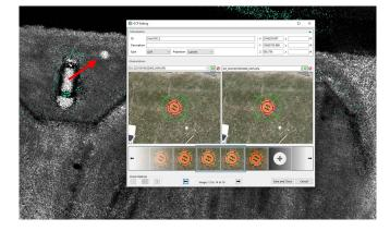
Correlator3D captures the XY value from the cursors position in the LiDAR generated Reference Ortho, and the Z value from the DEM.
