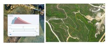
Automatically generated mosaics can be interactively adjusted. The mosaic editing module allows modifying seamlines with real-time visual feedback on the effect of changes. It can also be used for tuning the global mosaic colors and to enhance its appearance. Once editing is completed, the mosaic can be exported following a tiling scheme defined by the user.
