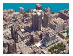
Correlator3D<sup>m</sup> can generate photorealistic 3D models. The process creates a mesh from a DSM, then uses input images to texturize it. The size of the output model is determined by the user.
