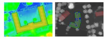
The feature extraction module enables the user to extract 3D features from a DSM by creating 3D polygons. Automatic contour detection of buildings and other features enable fast footprint collection. This semiautomatic design saves time over traditional vector extraction methods.
