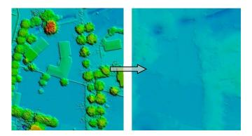
Through automatic filtering of the DSM, a DTM can then be extracted. The software analyzes the DSM and removes structures lying on the ground. DTMs are useful for generating orthophotos as they avoid visual artifacts (e.g. along building edges) caused by using DSMs.
