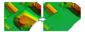
While automatically generated DSMs/DTMs are highly accurate, users may still desire to alter them for specific project requirements. The DEM editing module allows selecting a polygonal selection and performing operations such as crop/delete, set/offset elevation values and filter regions. A "Delete and Fill" function is also available for quick removal of structures.
