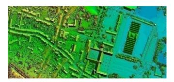
Once AT is done, a DSM can be generated at the output resolution specified by the user. During this process, overlapping regions between successive images are used as stereo data to derive elevation information. If required, a point cloud can also be produced in parallel during the same process.
