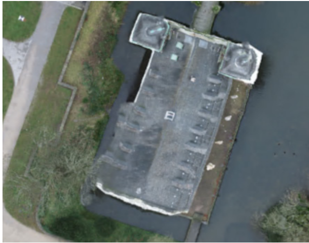
Figure 2a: True ortho from coarse DSM.
