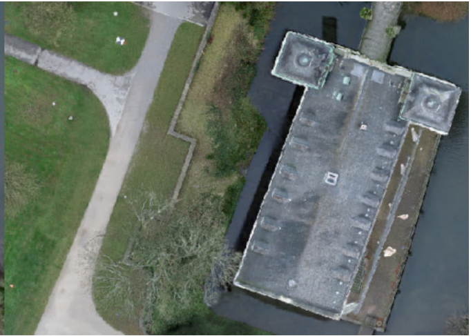
Figure 2b: True ortho from fine DSM.
