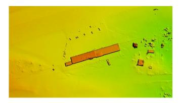
During this process, overlapping regions between successive images are used as stereo data to derive elevation information.
