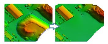
While automatically generated DSMs/DTMs are highly accurate, users may still desire to alter them for specific project requirements. The DEM editing module allows selecting a polygonal selection and performing operations such as crop/delete, set/offset elevation values and filter regions. A "Delete and Fill" function is also available for quick removal of structures.
