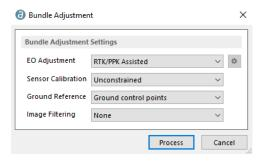
Bundle adjustment results should give an average tie point residual error smaller than 1 pixel. Higher residuals lead to inaccurate subsequent results.
