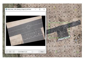
Before an orthomosaic can be generated, individual orthophotos must be created. Orthorectification consists of geometrically correcting the raw images such that they provide an accurate representation of the ground surface. The photos are thus adjusted for topographic relief, lens distortion and camera orientation. Once all orthophotos have been produced, they can be visualized through the software interface.
