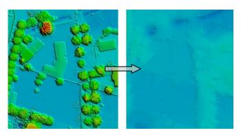
Through automatic filtering of the DSM, a DTM can then be extracted. The software analyzes the DSM and removes structures lying on the ground. DTMs are useful for generating orthophotos as they avoid visual artifacts (e.g. along building edges) caused by using DSMs.
