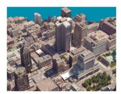
Correlator  $3D^{\text{TM}}$  can generate photorealistic 3D models. The process creates a mesh from a DSM, then uses input images to texturize it. The size of the output model is determined by the user.
