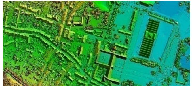
Once AT is done, a DSM can be generated at the output resolution specified by the user. During this process, overlapping regions between successive images are used as stereo data to derive elevation information. If required, a point cloud can also be produced in parallel during the same process.
