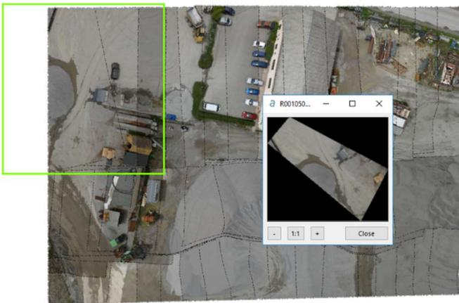
Before an orthomosaic can be generated, individual orthophotos must be created. Orthorectification consists of geometrically correcting the raw images such that they provide an accurate representation of the ground surface. The photos are thus adjusted for topographic relief, lens distortion and camera orientation. Once all orthophotos have been produced, they can be visualized through the software interface.
