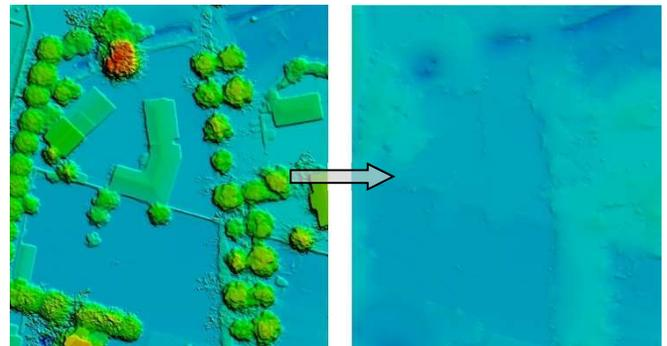
Through automatic filtering of the DSM, a DTM can then be extracted. The software analyzes the DSM and removes structures lying on the ground. DTMs are useful for generating orthophotos as they avoid visual artifacts (e.g. along building edges) caused by using DSMs.
