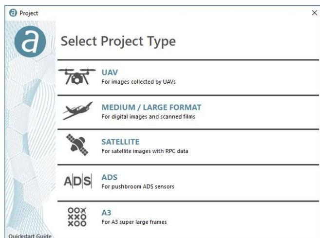
To assist in the creation of a new project, the software features a wizard to easily specify inputs. The user is first requested to select the type of data to be processed. Follow-up steps include specifying input images, camera and orientation parameters, as well as the projection.
