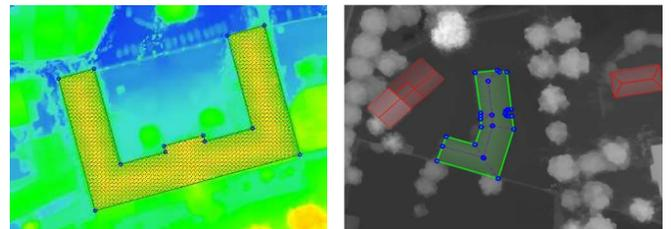
The feature extraction module enables to generate 3D features from a DSM by creating 3D polygons. It consists of a semi-automatic tool that can use photogrammetric / LiDAR DSMs and extract objects such as buildings, roads, waterbodies and forests.
