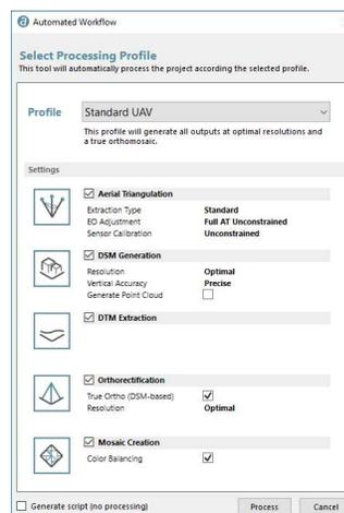
Once a project is created, the automated workflow can be used to automatically process the data according to the selected profile. Alternatively, users can perform all processing steps through the sequential use of individual modules. The latter approach is recommended for more experienced users and to achieve optimal results.
