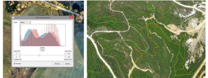
Automatically generated mosaics can be interactively adjusted. The mosaic editing module allows modifying seamlines with real-time visual feedback on the effect of changes. It can also be used for tuning the global mosaic colors and to enhance its appearance. Once editing is completed, the mosaic can be exported following a tiling scheme defined by the user.
